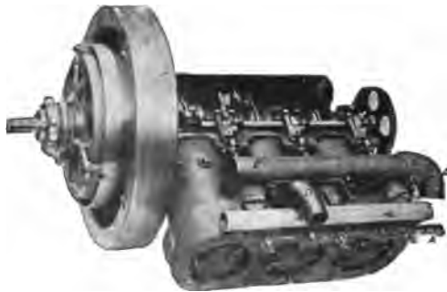
FIG 390. —The Duryea Three-cylinder 10 \frac{1}{2} B. H. P. Carriage Motor. A is the throttle slide, by which the gas supply to the three cylinders may be controlled by the combined steering and control lever shown in the last figure; B , single wire connecting anvils of the three sparking plugs in multiple, the other terminal of the circuit being connected to the middle parts of the cylinder; C , the common exhaust tube conveying the burned out gases to the muffler; D , the pipe conveying air to the jackets of the three cylinders.
